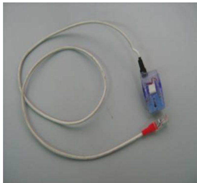
Fig. 1 The clip holding the diode and the phototransistor
