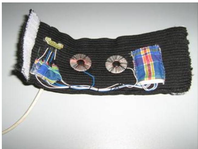
Fig. 3 Arm-band holding the temperature sensor and the electrodes.
