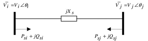
Fig. 8: Injection model of the UPFC
