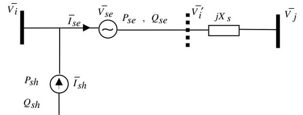
Fig. 3: Equivalent circuit diagram of UPFC
