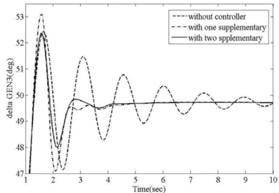
Fig. 16: Machine angle oscillation of GEN3 to three phase fault with one and two supplementary damping signals
