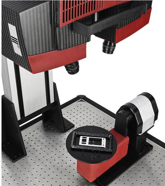
Fig. 4 Scanning process of model by using ATOS 3D optical scanning device with optional positioning device
