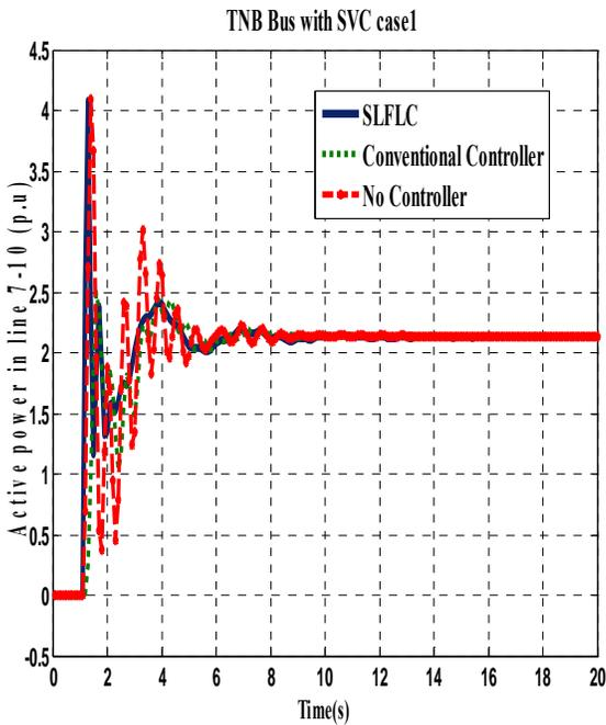
Figure 9 active powers in controlled line for line 7-10 outage
