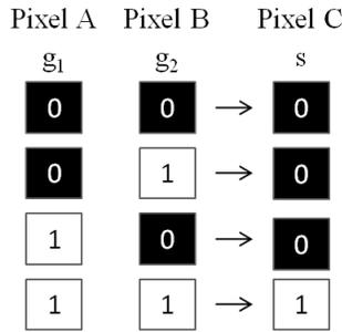
Fig. 1. Superimposing two binary pixels (which is the same as logical product of two pixels in Boolean algebra)
