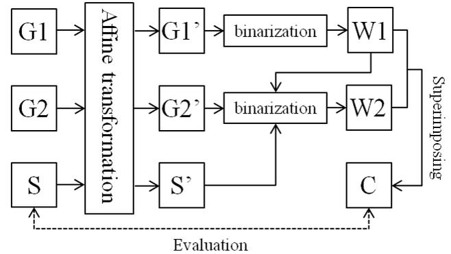
Fig. 3. The flowchart of Myodo's method
