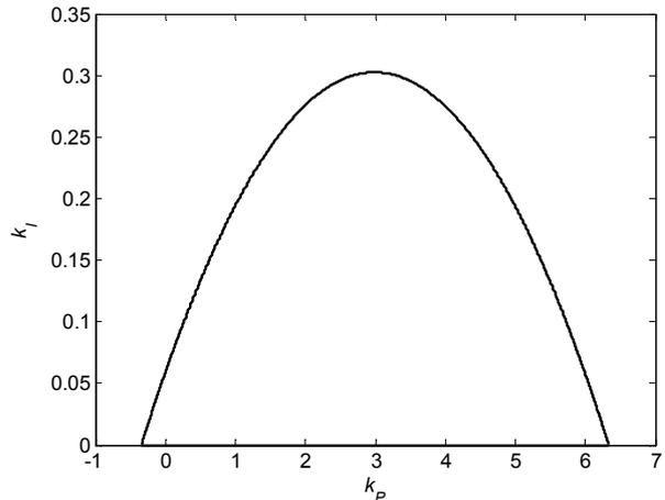
Fig. 5 stability region for system (29) and for  $k_D = 1$
