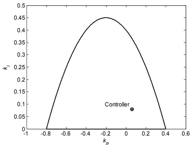
Fig. 3 position of the controller (22) in  $(k_p, k_I)$  plane
