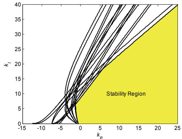
Fig. 9 stability region for the interval plant (42)
