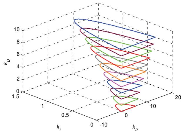
Fig. 6 stability regions for system (29) and for  $k_D \in \langle 0, 10 \rangle$
