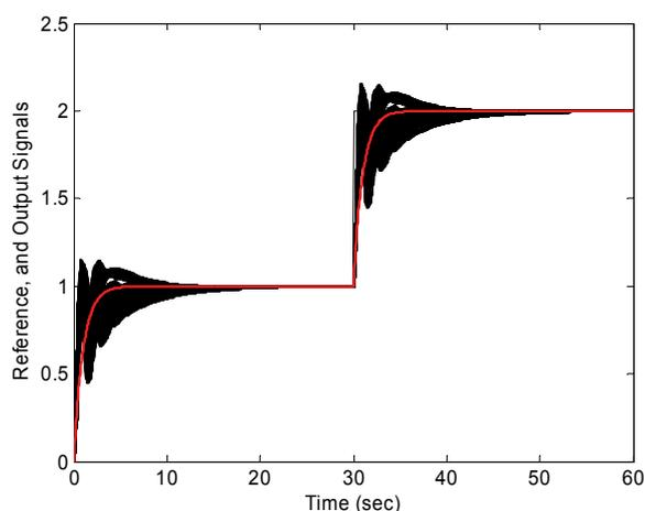
Fig. 10 output signals of 1024 “representative” plants and 1 nominal system
