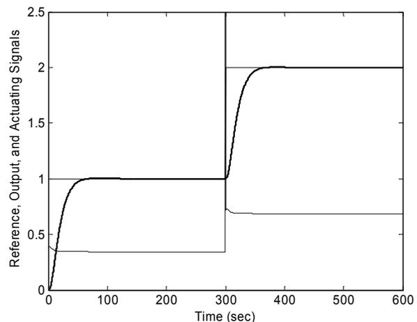
Fig. 8 control of plant (6) using PID controller (14)
