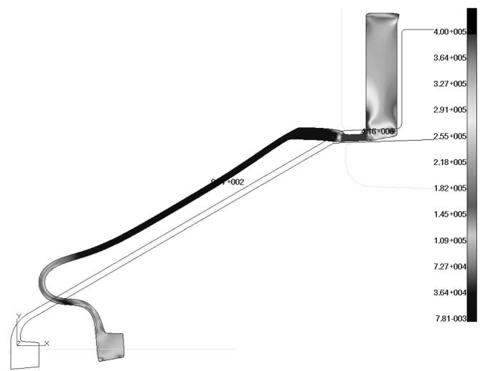
Fig. 21 final profile of the diaphragm II and its mounting to the basic position in valve – Von Mises stress [Pa]
