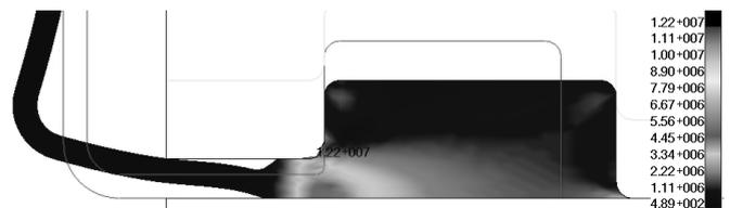
Fig. 7 results of initial design of diaphragm (after 2<sup>nd</sup> step) – Von Mises stress [Pa]
