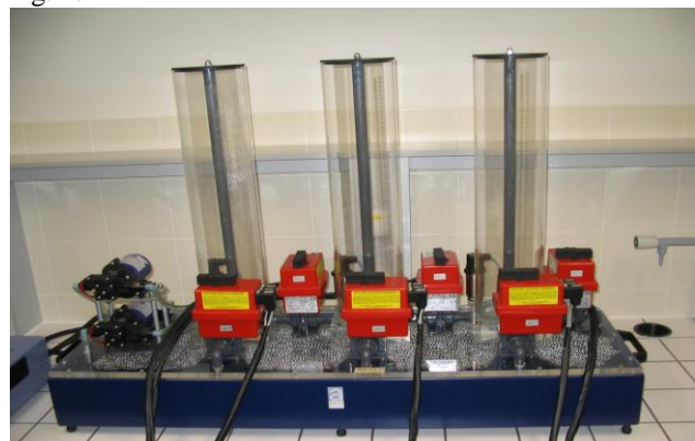
Fig. 1. Amira DTS200 – three tank system
