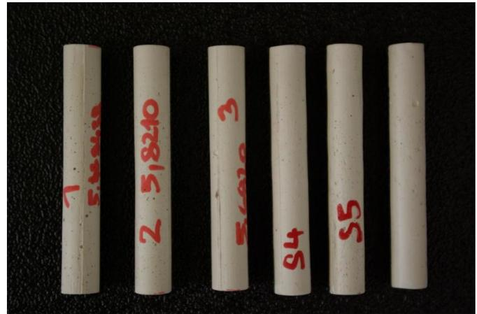
Fig. 4: Specimens prepared for creep tests.
