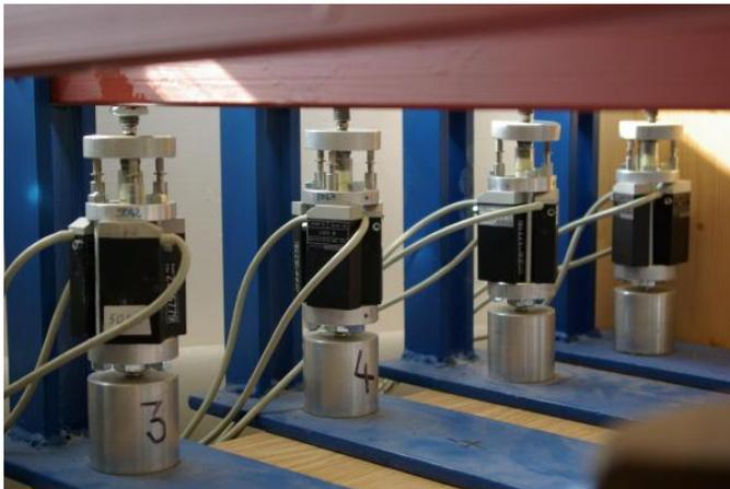
Fig.6: Lever mechanism – device for testing creep of homogenous materials.
