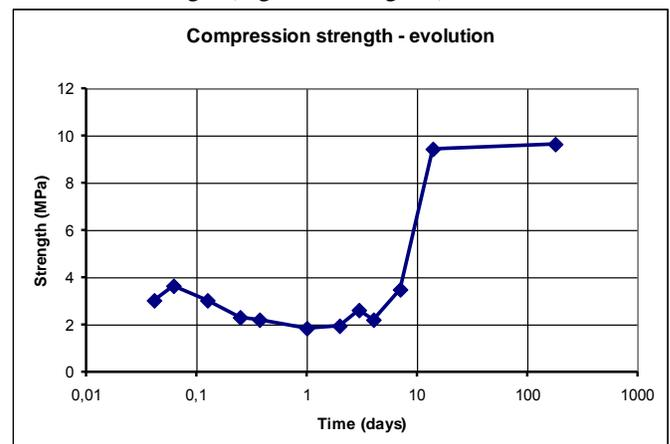
Fig.11: Compression strength and its evolution in time.
