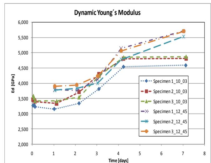
Fig.8: The time dependent changes of Dynamic Young's Modulus of chosen six specimens
