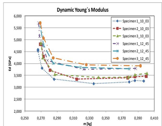
Fig.7: The changes of Dynamic Young's Modulus of chosen six specimens in dependence on weight of the specimens
