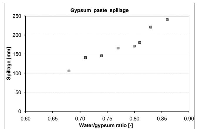
Fig. 1: Dependence of the gypsum paste spillage on a water/gypsum ratio
