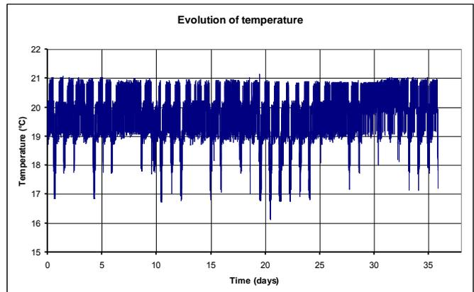
Fig.14: Temperature during the creep test.
