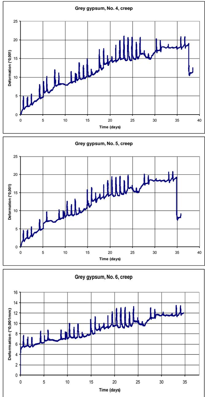
Fig.13: Creep of gray gypsum specimens.
