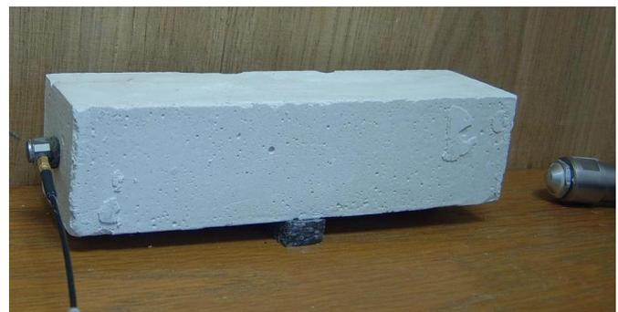
Fig. 3: The test arrangement for measuring the fundamental longitudinal resonant frequency of the gypsum specimen
