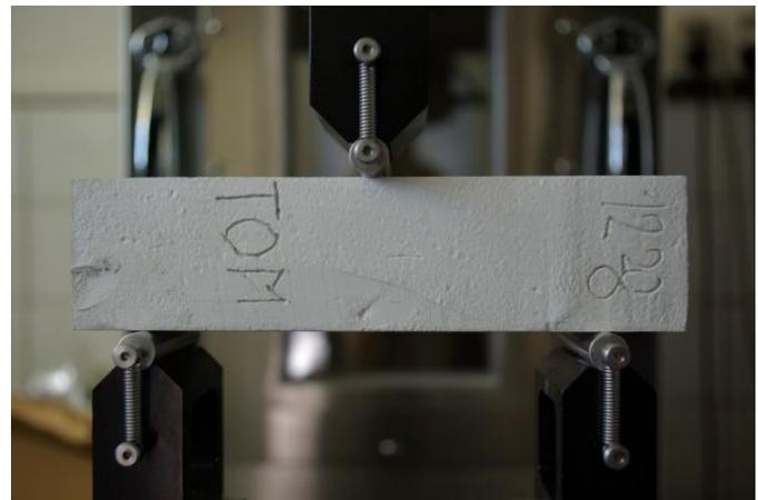
Fig. 5: Specimen in three-point bending test.
