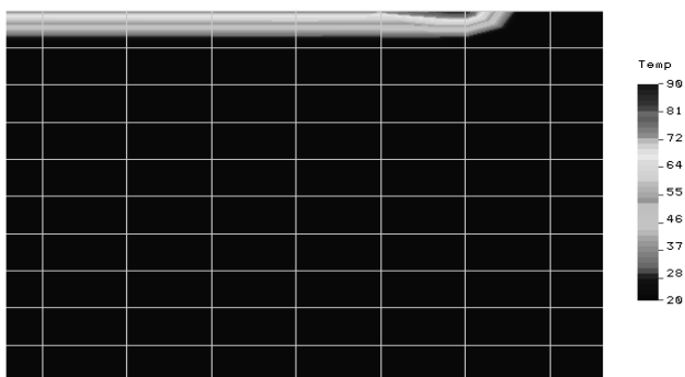
Fig. 23 2D simulation of the heat distribution in vicinity surrounds after 300 s. (speed 20 mm/s)
