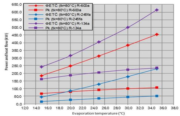
Fig. 9: Single phase heating pump at condensation temperature  $t_k = 80^\circ\text{C}$
