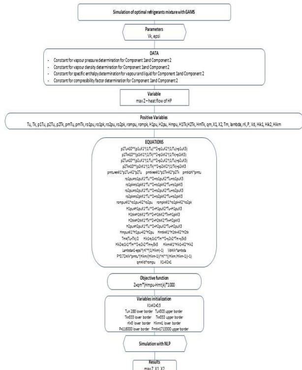
Fig. 3: Diagram for determining the optimal proportion of two agents in the mixture
