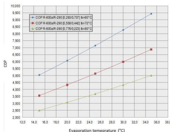
Fig. 5: Refrigerating number of the single phase heating pump with the optimal mixture proportion of R-600a and R-290
