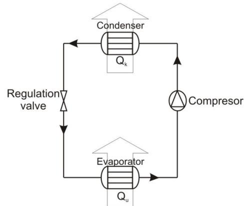
Fig 1: Single phase heating pump
