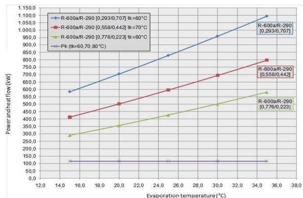
Fig. 4: Single phase heating pump with the optimal proportion of R-600a and R-290 in the mixture.
