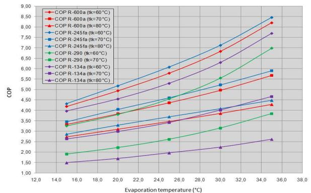
Fig. 10: Heating number of the single phase heating pump
